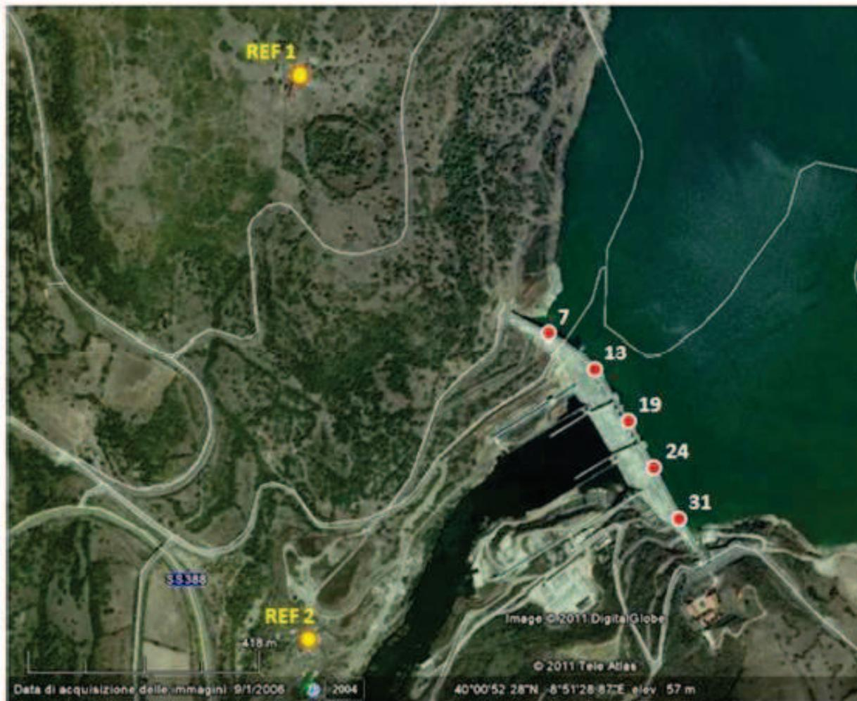
**Fig. 12. Cantoniera dam: the planned monitoring GNSS network**
